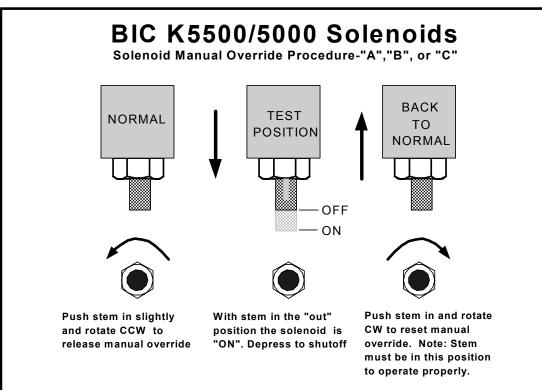
With attachment disconnected at quick couplers and engine running, the engine should pull down when the "C" solenoid is turned on. When the "C" and "B" solenoids are on at the same time there should be pressure at the left hand line (male QD). When the "C" and "A" solenoids are on at the same time there should be pressure at the right hand line (female QD).
