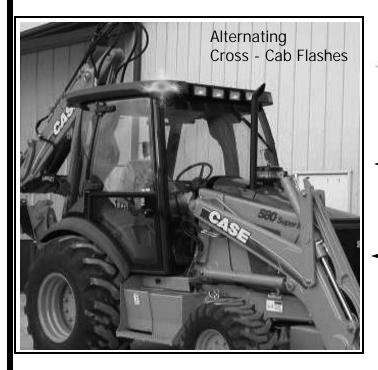
The BIC Four Corner Strobe Light Kit is an excellent safety addition that gives improved visibility in high traffic situations. This is a must have for government bids and machines that are frequently roaded.
