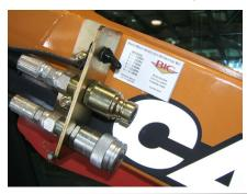
Parking brake must be set to operate hand held hydraulics.
